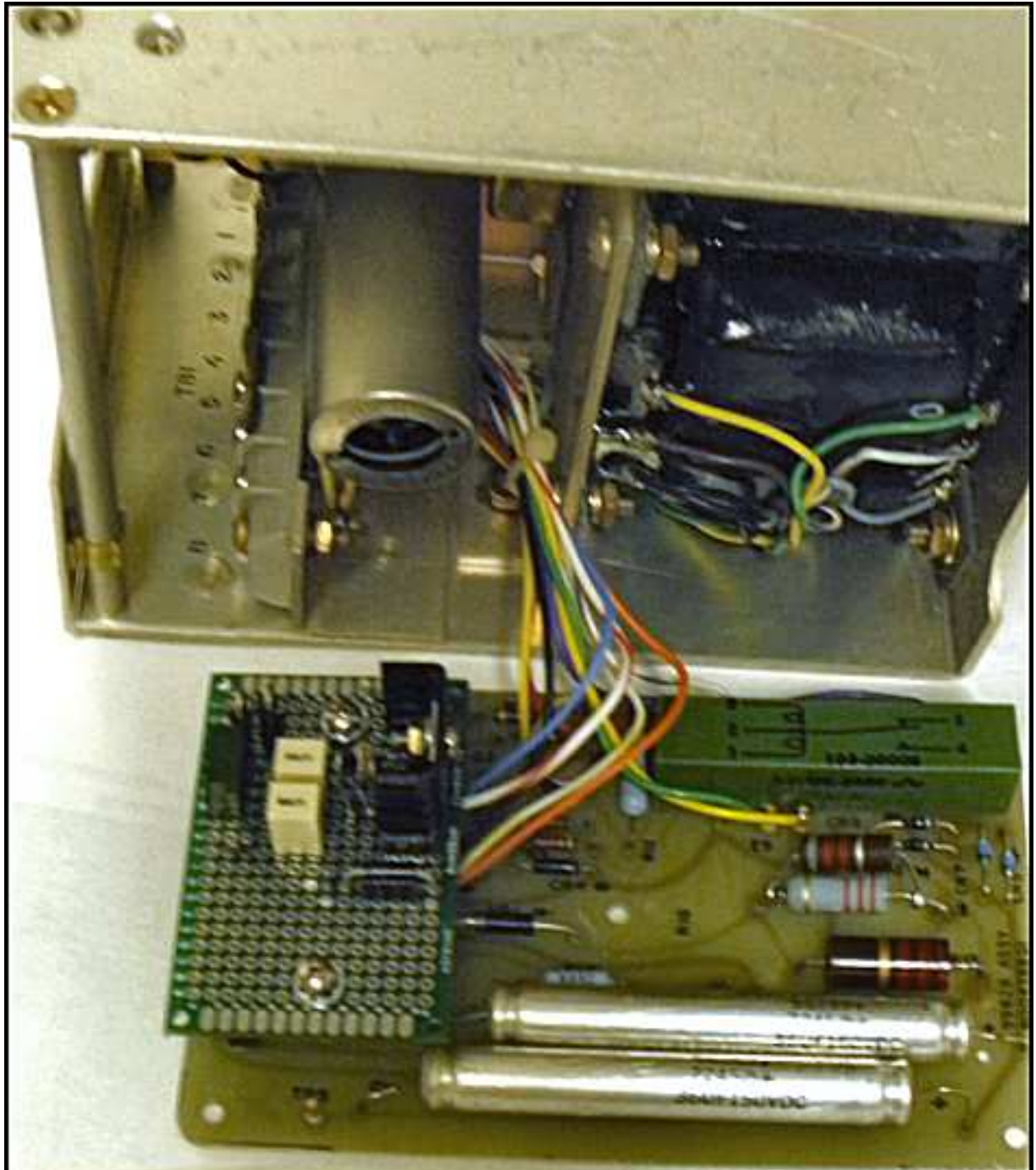
Bias board on carefully located standoffs ready for remounting in P.S. W1AN
